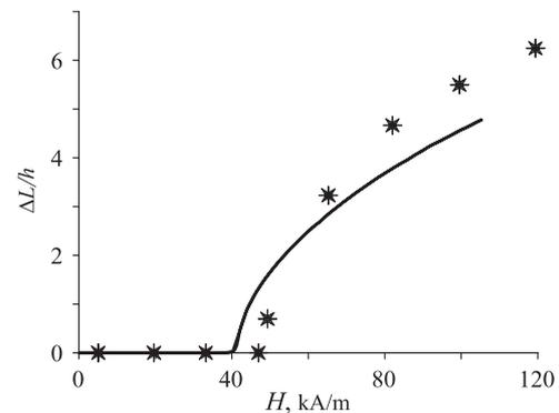
**Figure 4.** Theory versus experiment; the field dependence of the dome height for a membrane with  $D = 20 \text{ mm}$  and  $h = 1.9 \text{ mm}$ ; measurement (points) and modelling (solid line); the material parameters of the sample are  $\chi = 2.14$  and  $E = 30 \text{ kPa}$ .
