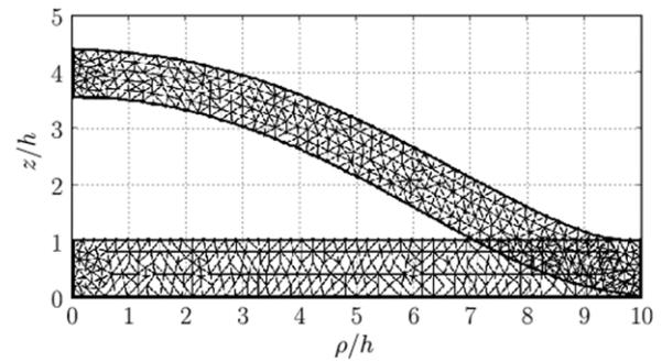
**Figure 2.** Profile of the axis cross-section of a membrane with  $\chi = 3$  and  $D/h = 20$  in the absence of the field (flat) and for  $H_0 \sqrt{3\mu_0/E} = 0.6$ .
