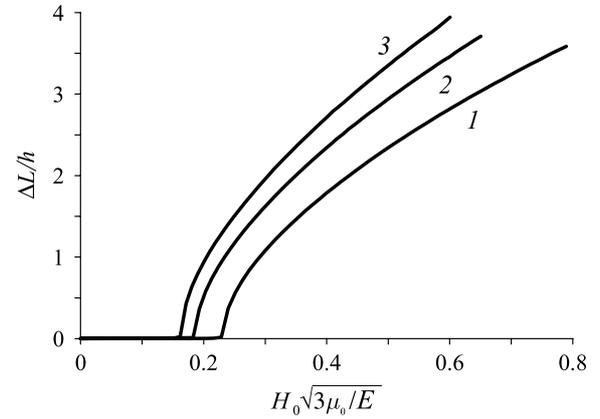
**Figure 1.** Dependence of the absolute value of the membrane central point displacement on the applied field strength;  $D/h = 20$ , magnetic susceptibility  $\chi = 2$  (1), 3 (2), 4 (3).
