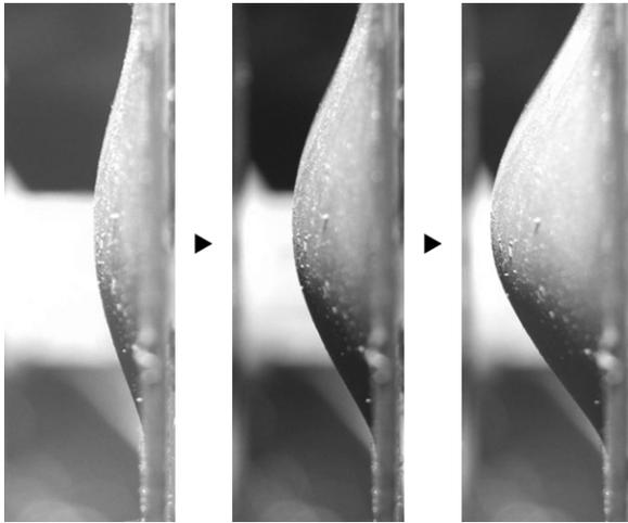
**Figure 3.** Domes formed by a membrane with  $D/h = 10$ ; left to right:  $H_0 = 50, 80$  and  $110 \text{ kA m}^{-1}$ .
